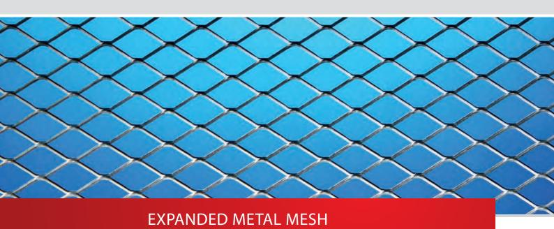
Expanded metal is a form of metal stock made by shearing a metal plate in a press, so that the metal stretches, leaving diamond-shaped voids surrounded by interlinked bars of the metal. The most common method of manufacture is to simultaneously slit and stretch the material with one motion. Expanded metal is also referred to as perforated metal. It is a large part of the metal industry and plays a key role in metal fabrication.
